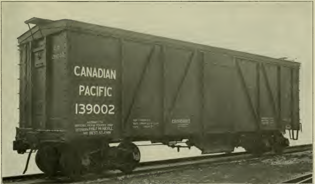
Hopper Bottom Box Car for Grain and Coal Traffic.
